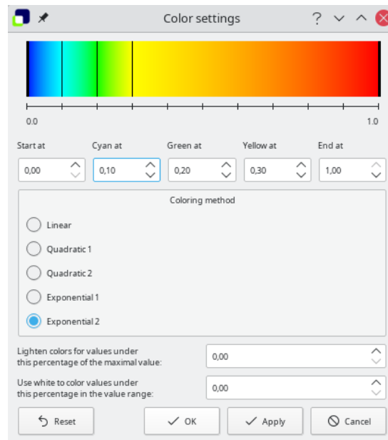
Figure 2.4: Configuration dialog of the default colormap which opened via the menu "Display => Edit colormap"
