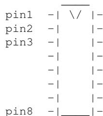
(This info comes courtesy of Hans-Christoph Wirth, and Juergen Exner, who posted it to [de.comp.os.linux.hardware](http://de.comp.os.linux.hardware)) You can solder a link between pin 3 and gnd, which will fix the mouse into MouseSystems mode.
