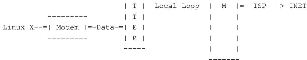
**Figure 2: DSL Splitterless (a.k.a. filtered) Block Diagram**
