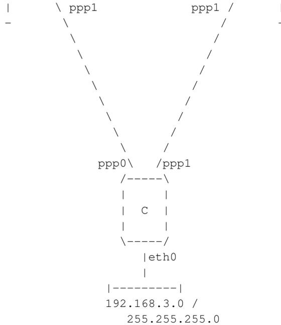
We have three routers A, B and C. Each router supports one ethernet segment with a Class C IP network (netmask 255.255.255.0). Each one also has a PPP link to each of the other two routers. The network ultimately forms a triangle.
